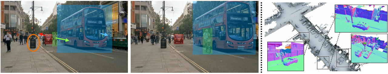
Figure 2: Research Thrusts. Dynamic Scenes (Left): Reconstructing monocular dynamic scenes with multiple moving objects (shaded in different colors), with unconstrained motions (arrows denote motions), and generalizing to novel object types (unseen trash can shape, circled) is still largely unsolved. Frames from video of a busy crosswalk. Generalization (Right): While past works can generalize well enough for static scenes to get a coarse reconstruction, they miss fine-grained details and glue distinct objects together (cars glued to the road). Figure from NKSr [10].
